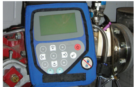
Biogas Flare and the associated testing equipment to track methane concentration
