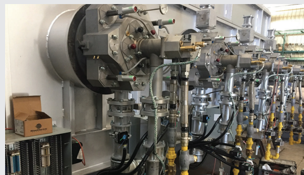
New Furnace with Regenerative Burners and Safety PLC Control
