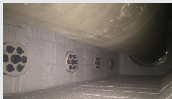
Inside new furnace: self regenerative flameless oxidation burners
