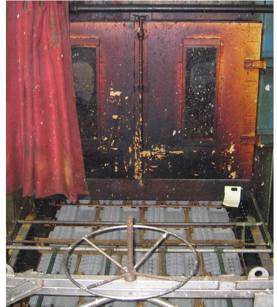
Dryer entrance showing hydrocarbon condensate
