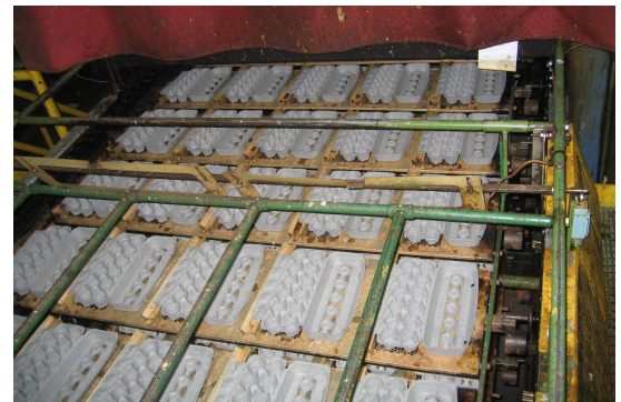
Mold release oil being applied to the cartons
