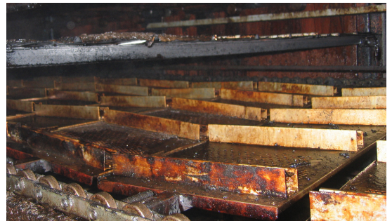
Carton conveyor inside the dryer
